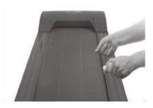
Pull up tightly of the running belt. Then put the silicone oil tor unning board. Then start the machine to running 3 minutes without loading. It is better to maintain like this every 30 hours working of the machine.
